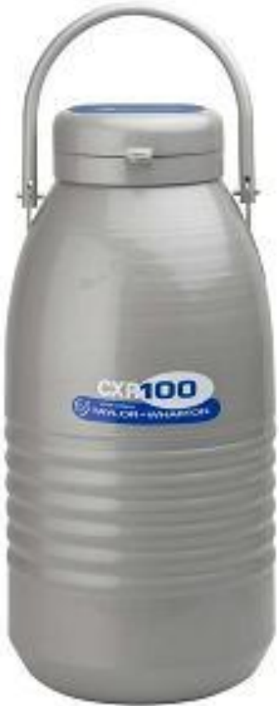
Dry shipper ( -150^{\circ}\text{C} ) (with liquid nitrogen in the walls)
